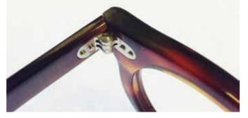
Using an electronic drill the hinges are joined together with specific screws.
