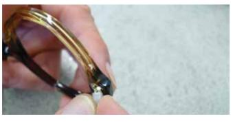
Frontals are next cleaned with a brush drill and an acetone bath. Then, before the tumbling process begins the hinges of each frame are capped with plastic hoods to ensure they are not damaged during the process.
