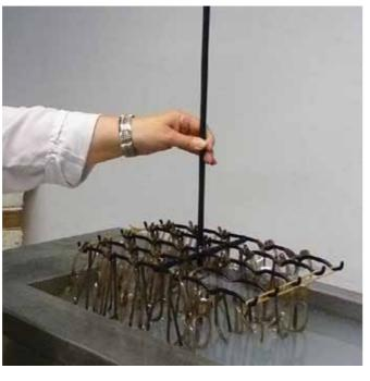
Once the third stage of tumbling is complete the frames are all removed and counted. They are then placed in an ultrasonic bath for three minutes at 30° and then left to air dry.
