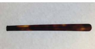
Temples are stamped out of 4mm acetate. A fustella, which is a cutter, is created like a cutter and using heat slices the temples out of the acetate. We currently have over 60 fustellas.
