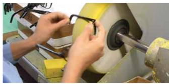
The frames are washed ultrasonically and once dried the frames are taken to the polishing room where a four step process of polishing begins.
