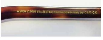
Once these details have been lasered onto the frame the graves are filled with gold ink and carefully polished to highlight the details.
