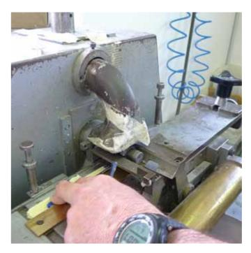
Once the temple has been shot it has its thickness reduced. As with the frontals we may only have 6mm acetate instead of 4mm which would be to thick and heavy to wear.
