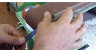
Resin is used to seal the logo within the grave, and then finally this is cleaned up by smoothing the excess resin away with a sanding belt.
