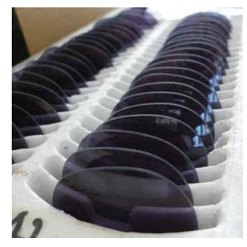
The main companies we currently use to glaze our frames are Zeiss, Dalloz and Intercast. It is very important to select lenses which are compatible with acetates as some materials such as polycarbonate can react with and crack the acetate when placed in one of our frames.
